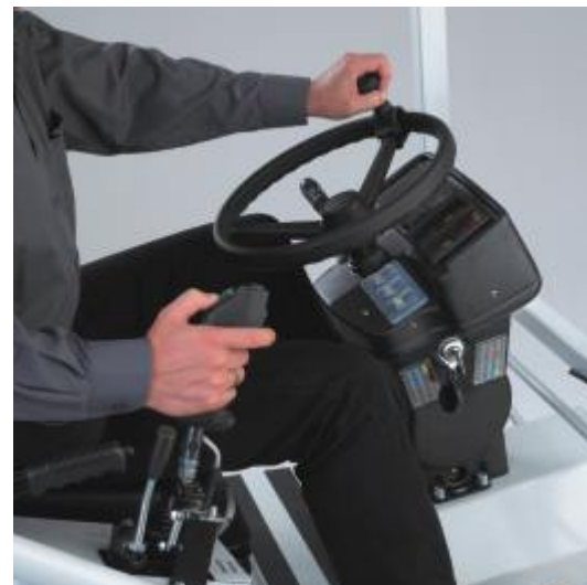
Effective control of the machine: steering with one hand while controlling the load arm and tools with the other.
