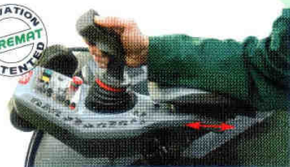
Single-lever LP mixed (elec. + hydr.) controls
