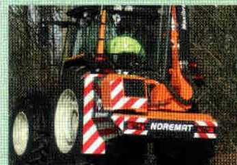
Tractor width indication kit
